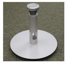
ATEX compliant and certified Safety Vent End-of-Line Flame Arrester on Vent Tube. Designed for use on tanks containing fuels. Stabiliser plate to keep upright in partially full flexitanks. 21/2"BSP Male connecting thread. Safety vent contains 5 layer element.
